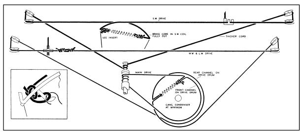
alignment with the gang spindle and the 52 metre mark is correctly aligned at maximum capacity.
