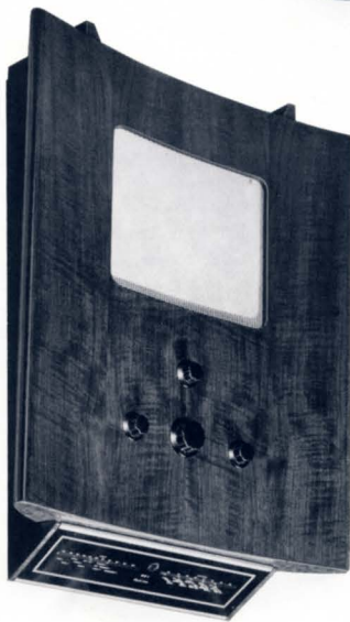
murphy A188C "Baffle" console. Seven-valve superet. Long and medium wavebands. Cabinet of American walnut with buff elm top panel. Magic eye tuning indicator. Push-pull output. Delayed A.G.C. Variable selectivity with four position tone control. Pick-up and extension speaker sockets. Frame aerial for local listening. PRICE £51 - 0 - 0 TAX PAID
